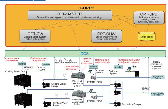
This solution U-OPT provides optimized "On Line Control" and "Guidance" for Utility Plant (Cooling towers, Various Type of Chillers, Pumps and Co-generation System, etc.) and then achieves CO2 reduction. This solution is Windows application and Various control systems (DCS, PLC system, etc.) can be easily connected with this solution through OPC (OLE for Process Control).
