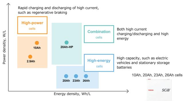
The SCiB™ rechargeable battery does not explode or ignite easily even when short-circuited, and lithium metal deposition is extremely unlikely to occur even under high input, low temperature, and long-term cycle use.
