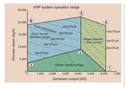
(Steam injection + additional burning) Area surrounded by (1), (4), (5) and (2) is for a (Steam injection + Additional burning) The increase of power generation in the right side of (2) and (5) area is by Steam injection to Gas turbine.
