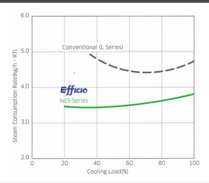
Cooling water inlet temperature conditions are as specified by the JIS standards (32°C at 100% load, 27°C at 0% load, with the temperature varying proportionally at loads between 0% and 100%).
